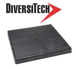
The Black Pad uses ground, recycled rubber in a coinjection process. The pad is extremely durable, resistant to ultraviolet light, and heavier than s completely plastic pad. Use 3 inch pads where local codes supercede the International code and require a pad thicker than 2".
